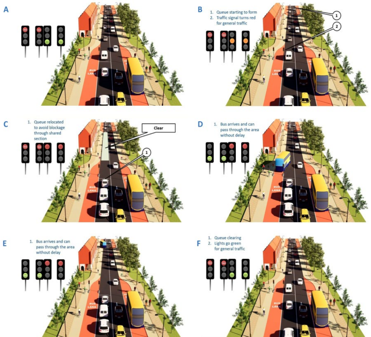
Image 4.10: Signalised Bus Priority Schematic Operation (Source: PDGB)
